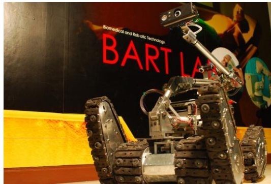
Fig. 1. The TeleOpIII, one of our two tele-operative robots in BART LAB Rescue team. The TeleOpIII employs tracked locomotion system with 4 independent flippers, and equips with an inverse-kinematically controlled manipulator to enhance more ability to search and retrieve better victim information, similar to other robots in [1,2]
